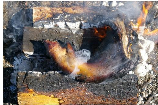
**Figure 10:** *Specimen 1. Specimen temperature: 379°C. Fire temperature: >900°C. Time: T+23. Efford 2016.*
