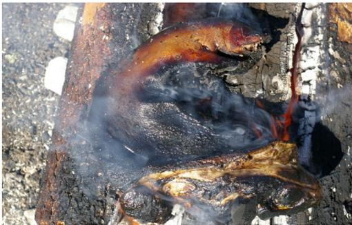
**Figure 13:** Specimen 2. Specimen temperature: 553.9°C. Fire temperature: >900°C. Time: T+39. Efford 2016.
