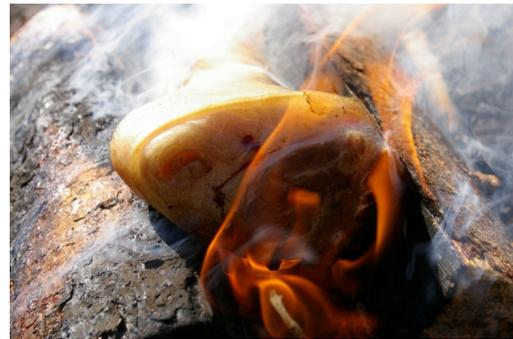
**Figure 6:** *Specimen 1. Specimen temperature: 235.6°C. Fire temperature read >900°C. Time: T+14. Efford 2016.*
