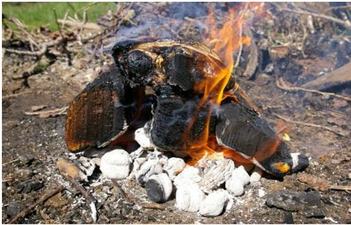
**Figure 7:** *Specimen 2. Specimen temperature read 259.5°C. Time: T+10. Efford 2016.*
