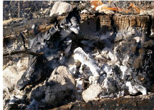
**Figure 14:** Specimen 2. Specimen temperature: 649.1°C. Fire temperature: >900°C. Time: T+69. Efford 2016.
