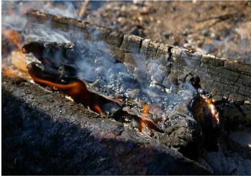
**Figure 11:** Specimen 1. Specimen temperature: 502.7°C. Fire temperature: >900°C. Time: T+30. Efford 2016.
