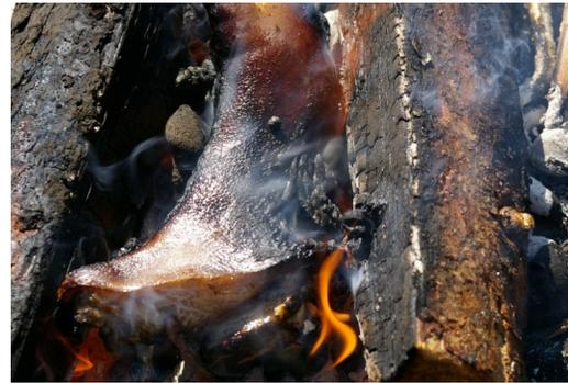
**Figure 12:** Specimen 2. Specimen temperature: 480.2°C. Fire temperature: >900°C. Time: T+24. Efford 2016.
