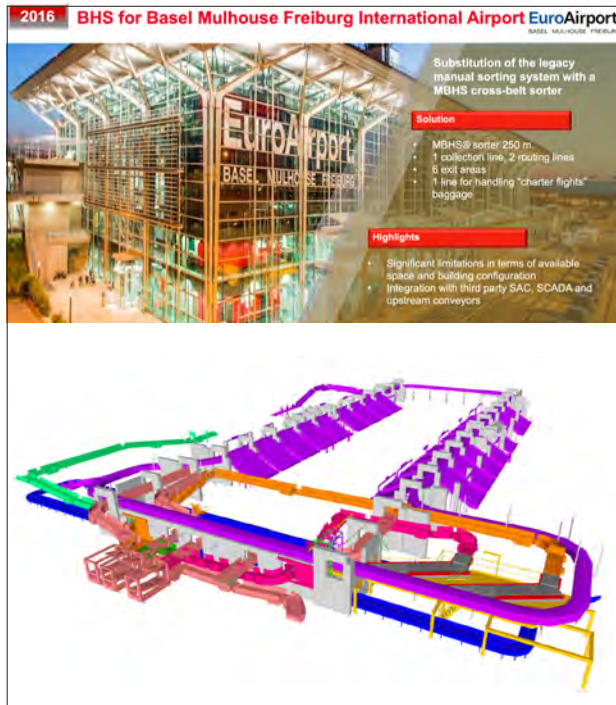
Figure 4. Automatic Cross-belt Sorter (Baggage Handling System) for Basel-Mulhouse Airport. Sources: Alstef Group (2016); EuroAirport (2024).
