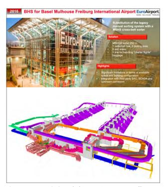
Figure 4. Automatic Cross-belt Sorter (Baggage Handling System) for Basel-Mulhouse Airport. Sources: Alstef Group (2016); EuroAirport (2024).
