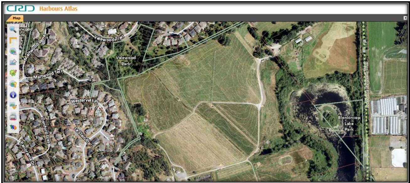
FIGURE 9. CRD ATLAS TOPOGRAPHICAL MAP OF PROJECT AREA, THE WHITE LINES INDICATE A ONE METER DROP IN ELEVATION. MAP CREATED JANUARY 4, 2016.
