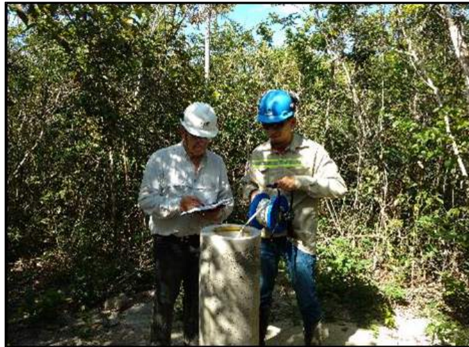
Picture 2: Water level measuring
