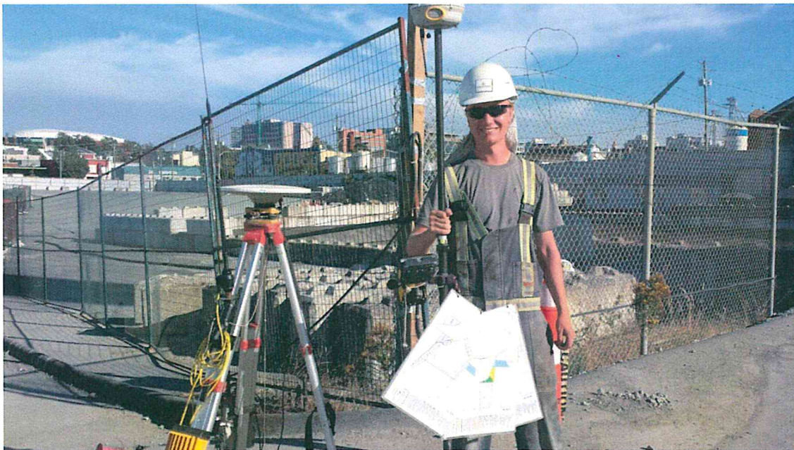
Figure 4: Trimble SPS GPS system and layer maps
