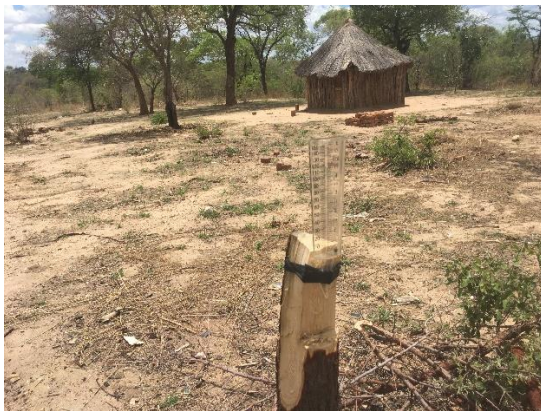
Figure 12: Rain-gauge set up near Siandwazi dam
