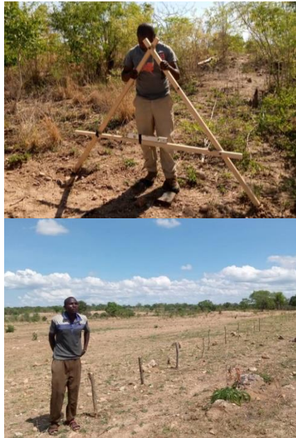
Figure 10: a) Maambo (Ministry of Agriculture) next to an adapted A-frame which uses a level to establish two points of equal elevation to build a contour; b) contour for farmers to follow while tilling
