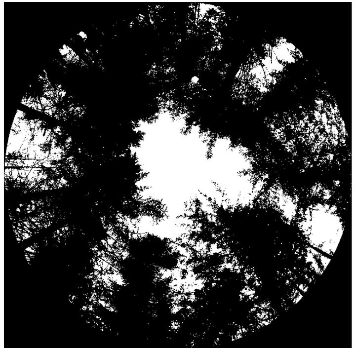
*Figure 6: Binarized Image created with Gap Light Analyzer program*
