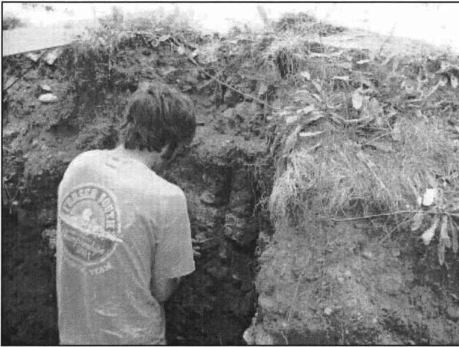
Figure 2 (above). Carving a space around the block using a soil knife courtesy of Chris Springer (Photo by author).
