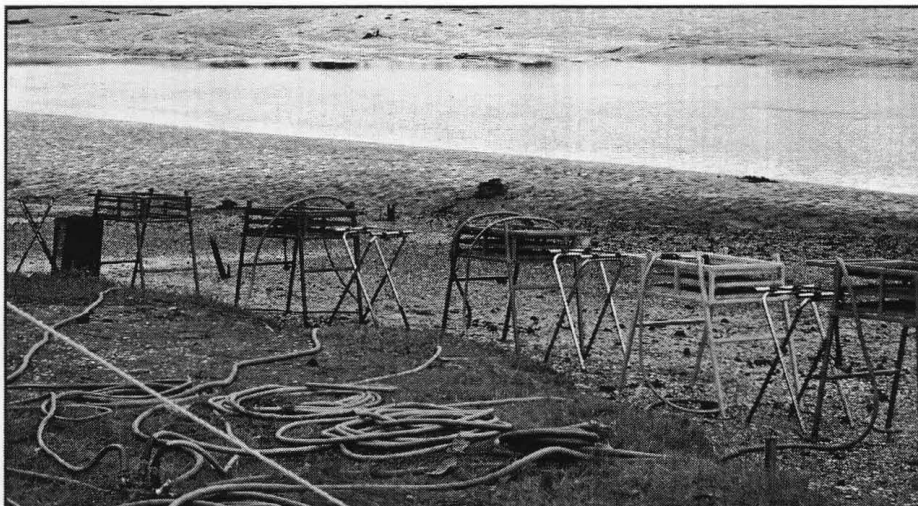
The metal screens developed by the welding department of the South Puget Sound Community College. Each screen has 3 layers of differently gauged screens ranging from 1/2-inch to 1/8-inch.
