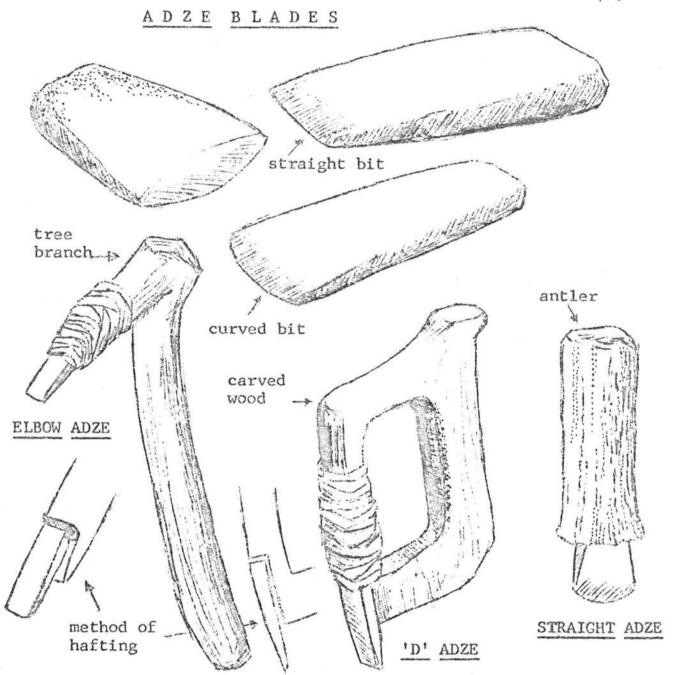
THE ADZE, in all its variations, formed part of the triad of the major woodworking industry along most of the Pacific Northwest Coast; the handmaul and the wedge being the two other important tools. The stone used for the blade of the adze had to be extremely hard and durable, and capable of taking a sharp edge that could be resharpened with an abrasive stone.
