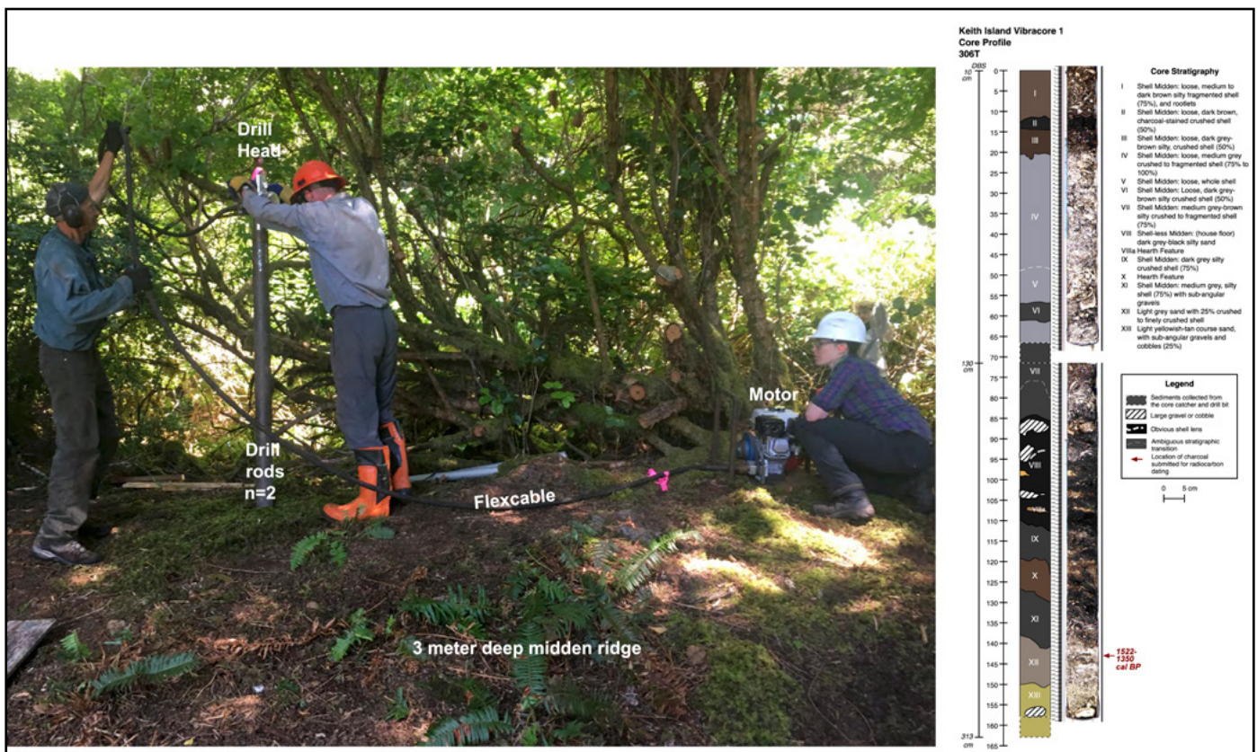
Figure 1. Right: Vibracoring at Kakmakimilh (Photo: Iain McKechnie). Left: Keith Island 1 profile drawing, GSC core photograph, radiocarbon sample locations and date ranges (cal BP) and description of core stratigraphy.
